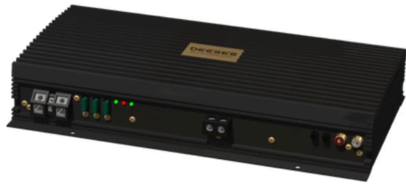
The BS-0 series is designed to deliver a powerful and impressive sound experience through high-quality passive and semiconductor components, along with an innovative design philosophy. With wide frequency response, low distortion, and high efficiency, it integrates seamlessly into in-car audio systems. Its compact structure allows for easy installation in various setup scenarios.
